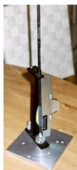
Tool used to stick [vanes](#) on the shafts of the [arrows](#) with precision.
